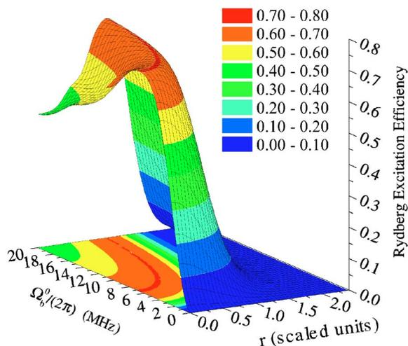
FIG. 4. (Color online) Efficiency of the Rydberg-state excitation,  $\eta_a$ , vs the central Rabi frequency of the upper transition,  $\Omega_b^0/(2\pi)$ , and distance  $r$  from the center of the blue beam. The Rabi frequency of the lower transition is 10 MHz.
